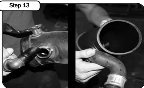
Step 13 1. Remove crank case breather from factory tube. 2. Place rubber grommet into hole and press crank case breather into grommet on tube.
