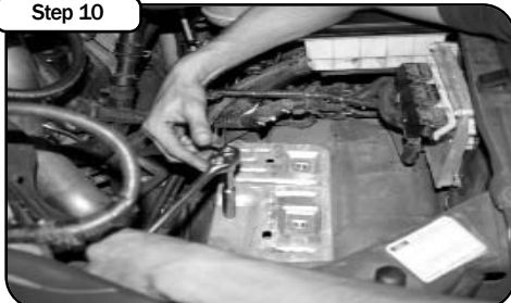
Step 10 Remove battery tray support bracket from vehicle using a 13mm socket or wrench.
