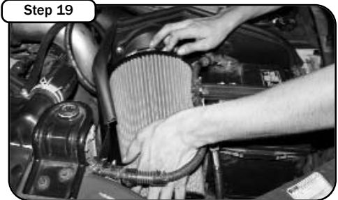
Step 19 Install filter onto tube. Tighten clamp.
