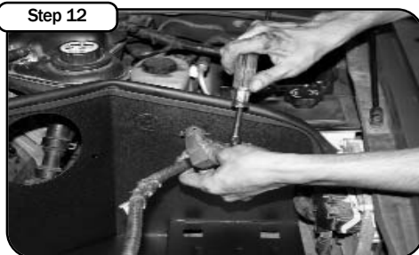
Step 12 Install rubber grommet onto housing. With both batteries disconnected remove wire from terminal using a 10mm socket and pull wire through housing and reconnect.
