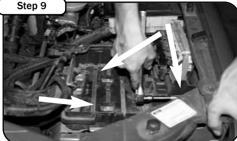
Step 9 Using a 13mm socket or wrench Remove all screws holding the battery tray in the vehicle.
