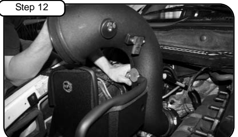
Install hi-temp coupler with clamps provided to tube. Now install tube into vehicle.
