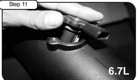
6.7L, remove MAF sensor and install to new tube with screws and gasket ( Make sure gasket is between sensor and tube ) Install grommet ONLY to tube.
