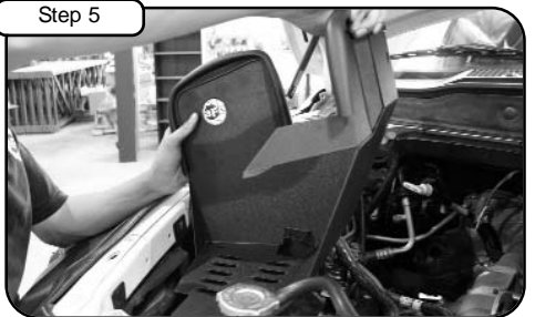
Install 3/4" Trim seal to housing. Now install housing into vehicle.
