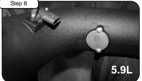
With T-20 torx bit remove temp sensor and ( with gasket and screws provided ) install into new tube. ( 5.9L place MAF cover with gasket and tighten using short screws provided.)
