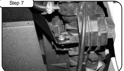
Use M6 screw/nut and washer and tighten housing to bracket "D" and tighten.
