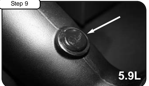
5.9L install urethane plug to hole on tube.
