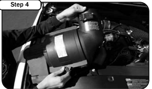
Gently pull out whole airbox. Grab from MAF area, (not directly on MAF) and pull up. It is held in place with rubber grommets. Remove the airbox mounting plate bracket.
