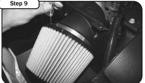
Carefully install the 6" aFe air filter and tighten with 5/16 nut driver.
