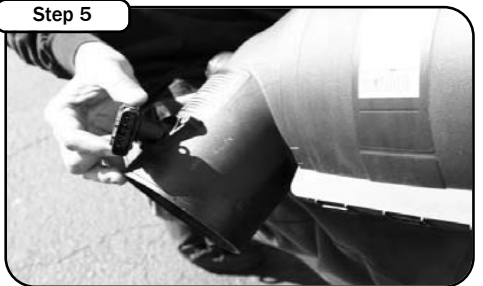
Take out factory MAF sensor using the torx T-20 bit to unscrew bolts. Be careful in handling the MAF sensor.
