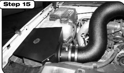
Step 15 Place the included CARB EO Sticker on or near the intake system on a smooth, clean surface. E.O. identification label is required in passing the Smog Check Inspection. Complete Stage 2 kit installed. Make sure all clamps are tight and all components are secure. Check and retighten connections and filter after a few hours of operation.
