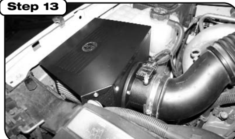
Step 13 Complete Stage 1 kit installed, for Stage II kit and Torque Booster Tube instructions, continue on to step 14 and 15.
