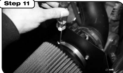
Step 11 Install filter and tighten clamp. Do not use oil or grease.
