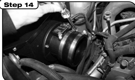
Step 14 Install provided couplers. Be sure to install the small end of the tapered coupler to the turbo inlet housing. The remaining coupler must be installed with the smaller inner diameter attached to the heat shield, and the larger inner diameter will receive the Stage II tube. Install Stage II tube into couplers. Reposition duct clamps if additional clearance is necessary.
