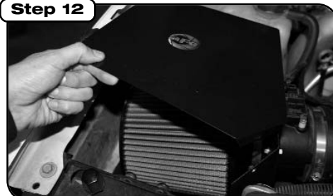
Step 12 Place cover on top of housing and fasten securely using 3 supplied 1/4-20x3/4 bolts and washers. For stage I kits, make sure all clamps are tight and all components are secure. Check and retighten connections and filter after a few hours of operation. (End of stage I installation instructions.)
